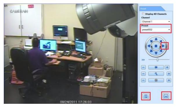
6. Go back to the main camera live screen and select Preset 101 and click on Enter button to start moving the camera from left to right and back and forth.
